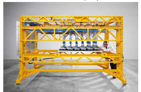
CFV Solar puts new mechanical load test stand into operation
